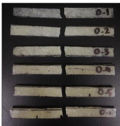
Figure 16: Fractured sample of DW/epoxy with different ratio, (A) Ratio of 0.1 DW, (B) Ratio of 0.2 DW, (C) Ratio of 0.3 DW, (D) Ratio of 0.4 DW, (E) Ratio of 0.5 DW, (F) Ratio of 0.6 DW
