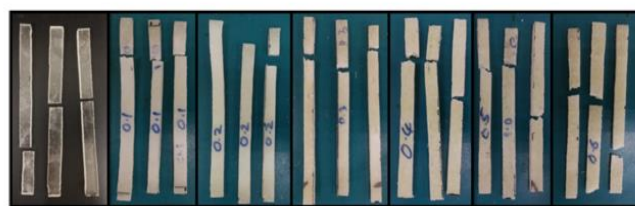
Figure 12: Physical properties of the tensile strength sample after tested; (A) Control Sample, (B) Ratio of 0.1DW, (C) Ratio of 0.2 DW, (D) Ratio of 0.3 DW, (E) Ratio of 0.4 DW, (F) Ratio of 0.5 DW, (G) Ratio of 0.6 DW
