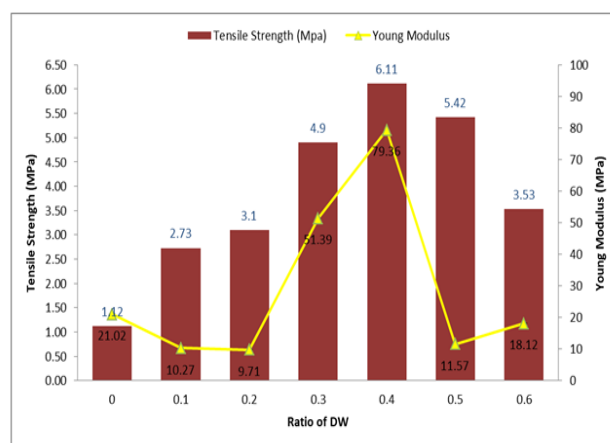
Figure 11: Tensile properties of DW/epoxy composites
