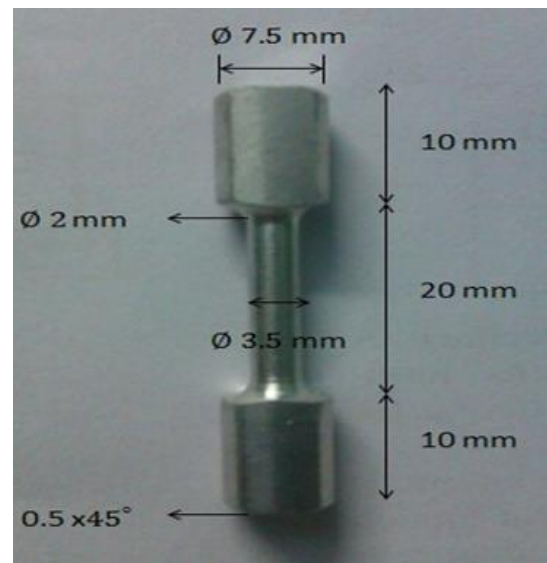
Figure 6: Torsion testing specimen with flattened grip
