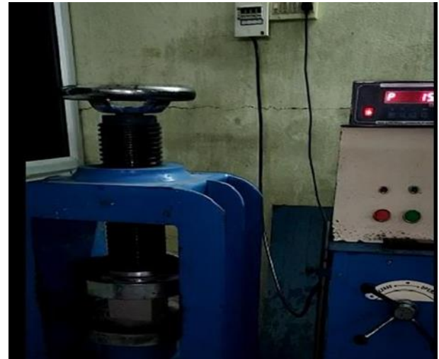
Fig 4. Application of load in CTM
