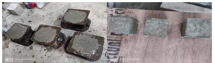
Fig 1 Casting of concrete cubes
