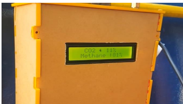
Figure 9. Percentage of Methane and Carbon Dioxide display on LCD
