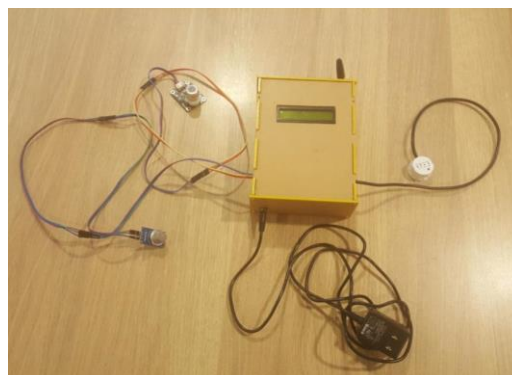
Figure 4. Methane Production Monitoring System and Overfeeding Notification
