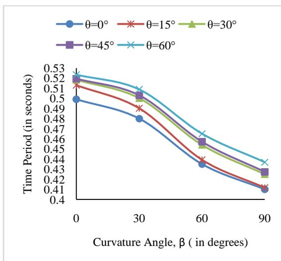
a. Variations in time periods of 1<sup>st</sup> In-Plane Mode for various bridge configurations
