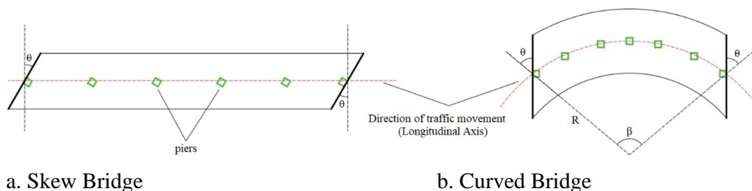
Figure 1. Schematic Diagram for Skew Bridge and Curved Bridge
