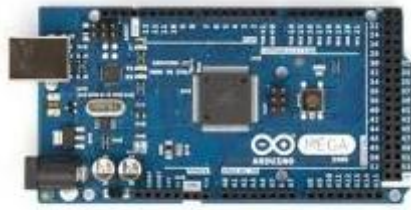
Fig 4: Arduino compatible ATMEGA2560
