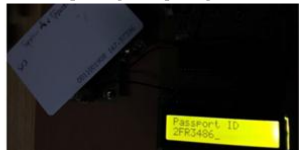
Fig 5.5 Passport Id of passenger is displayed when Tag is swiped
