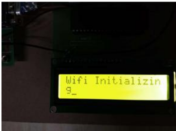
Fig 5.2 Initialization Status displayed in LCD.
