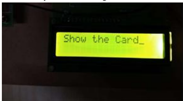
Fig 5.3 LCD Message Indicating The System Is Ready To Read The Tag.
