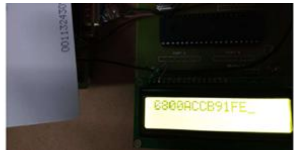
Fig 5.4 RFID Tag code being displayed when passenger swipes tag.
