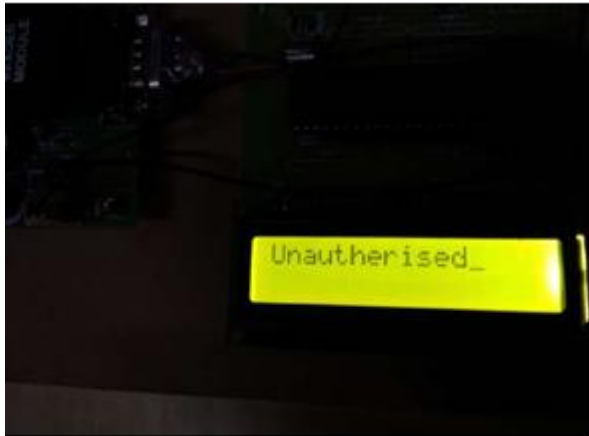
Fig 5.7 “Unauthorized” is displayed in the LCD when a blocked/unidentified tag is swiped
