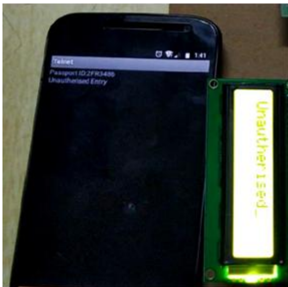
Fig 5.8 “Unauthorized entry” is displayed at the authority's screen (PHONE) when a blocked/unidentified tag is swiped.
