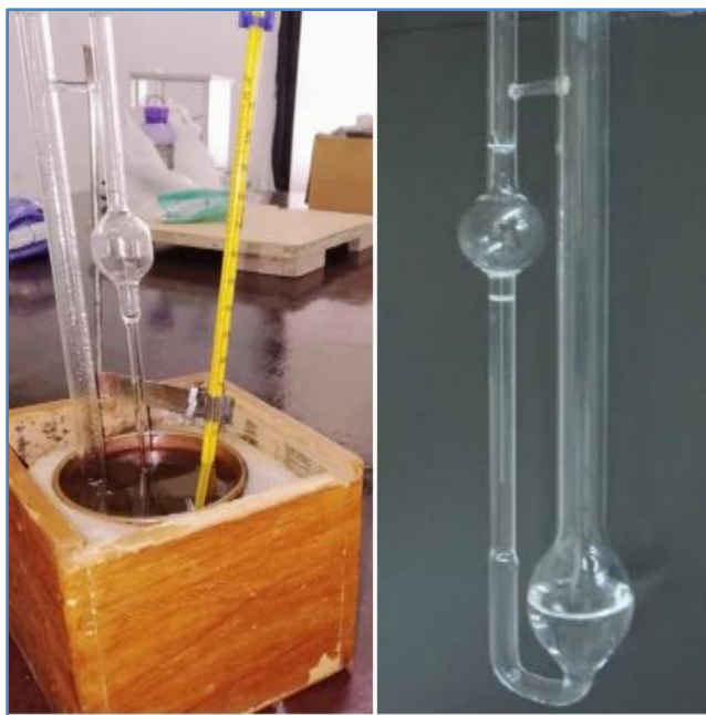
Fig.2. Viscosity measurement by Ostwald's viscometer
