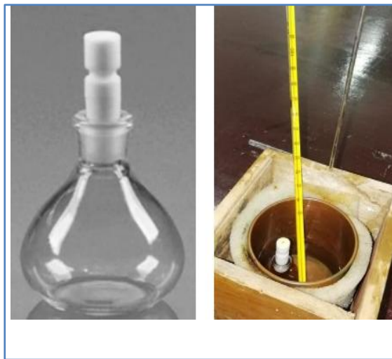
Fig.1. Density measurement by Pycnometer
