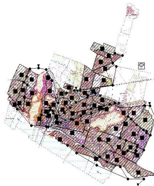
Fig 3: Discretization of sub catchments in SWMM.
