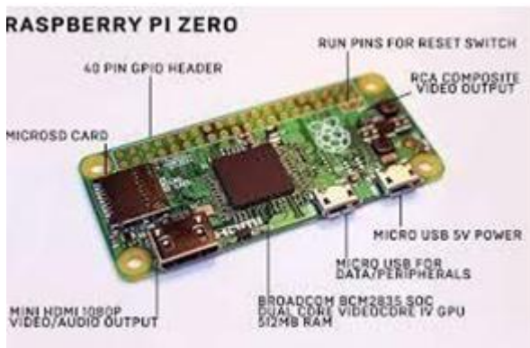
Figure 1.3: Raspberry pie zero
