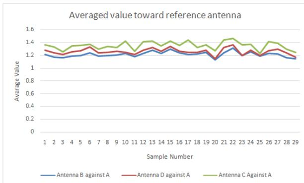
Figure 7: Amplitudes of antenna B, C and D is divided with amplitude of Antenna A to obtain average value
