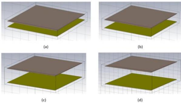
Figure 1: The gap is 30mm for Antenna A (a), 50mm for Antenna B (b), 100 mm for Antenna C (c) (all dimensions is 420 mm × 297 mm × 1.6 mm) and 100 mm for Antenna D dimensions of 190 × 190 mm × 1.6 mm (d).
