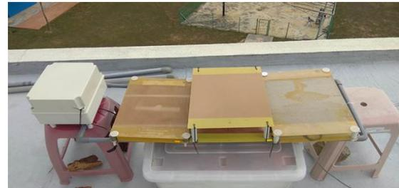
Figure 2: Constructed antennas placed on a PVC rack and stool. From the left: Antenna D with 100 mm gap with smaller area (antenna inside box), Antenna A with 30 mm gap, Antenna C with 100 mm and, Antenna B with 50 mm gap.
