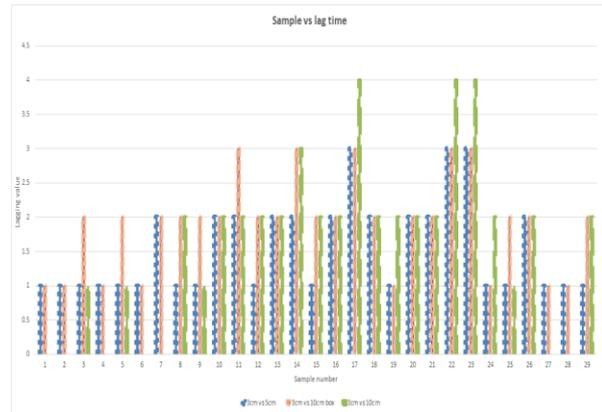
Figure 8: Cross correlation method is applied to all the selected return stroke waveform. Blue dotted line represents 50 mm air gap averaged out to reference, Brown double dash lines represents 100 mm air gap averaged to reference and green long dash lines represent 100 mm air gap averaged out to reference.
