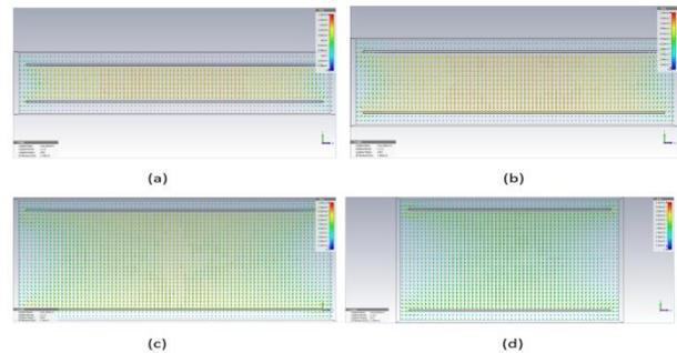
Figure 5: Direction of electric field for simulation results of parallel plate capacitive antenna with different air gaps spacing. (a) Antenna A with 30 mm air gaps (b) Antenna B with 50 mm air gaps (c) Antenna C with 100 mm air gaps (d) Antenna D with 100 mm air gaps with smaller area.
