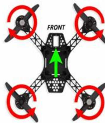
Figure 3: Schematic diagram of the four rotors on a UAV.
