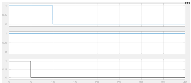
Figure 17: trip signal of circuit breaker
