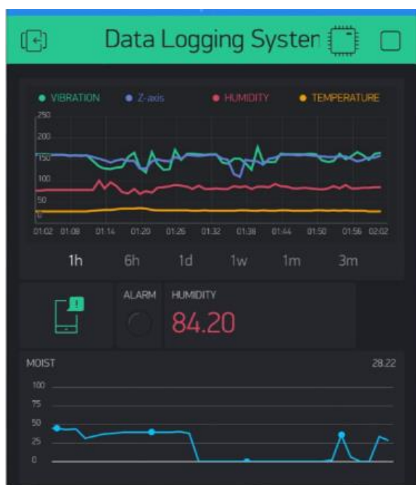
Figure 8.0: landslide data as displayed through smartphone application
