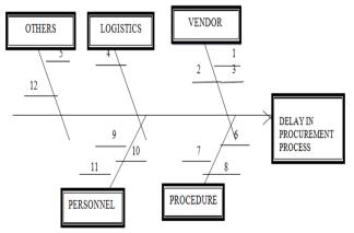
The above diagram shows the factors such as procedure, personnel, vendor, logistics, others etc. which affect the overall problem at CE. Smaller arrows connect the sub-causes to major
