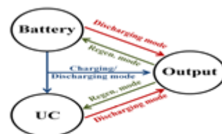
Fig. 2. Operation modes of the MIC
