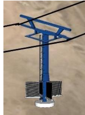
Figure 14. Turret implemented with four fog collectors and a water storage tank.
