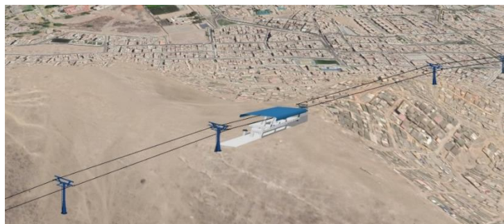
Figure 8. Intermediate station: Located at one or more points between the two endpoints of the system. The stations offer additional opportunities for passengers to board and get off a system. [10]
