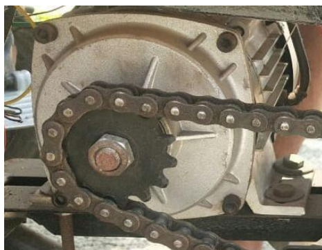
Figure 2. BLDC motor drive with chain attachment
