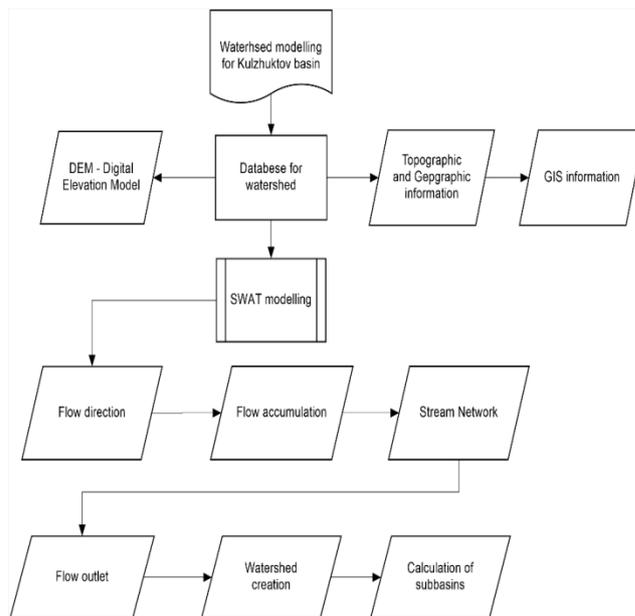
**Figure 2. Image Methodology for the creation of a temporary stream basin model on the southern slopes of the ridge**
