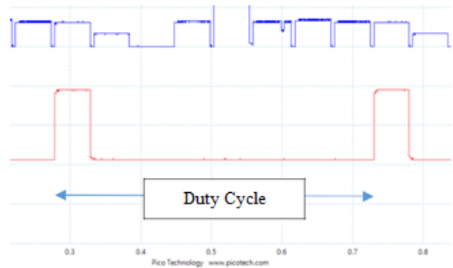
Figure 10: Duty cycle for Single Frame
