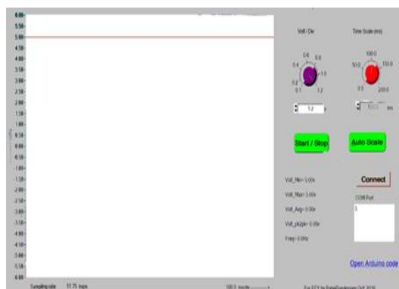
Fig.8 shows dc line when connected to 5V in the Arduino board
