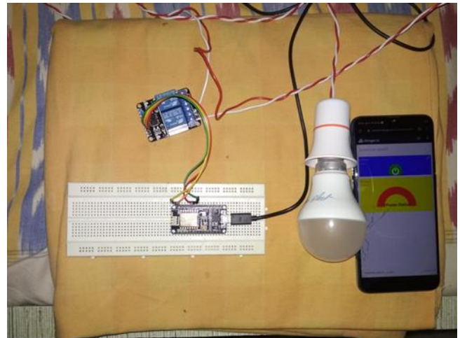
Figure 10 Working of Thingier.io in circuit OFF condition
