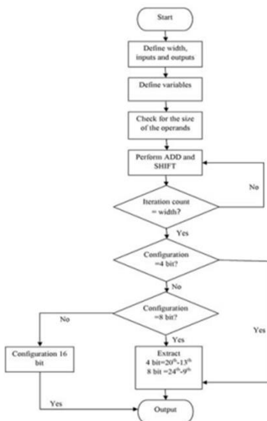
Fig.2. Reusable booth multiplier with the concept of configuration registers on the flow chart
