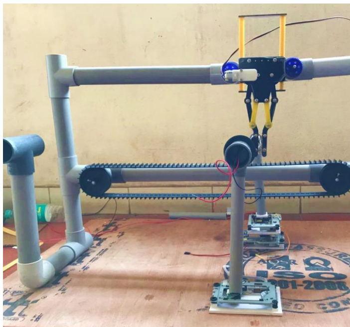
Fig. 8 Prototype of a Semi-Automatic Flower Tying Machine
