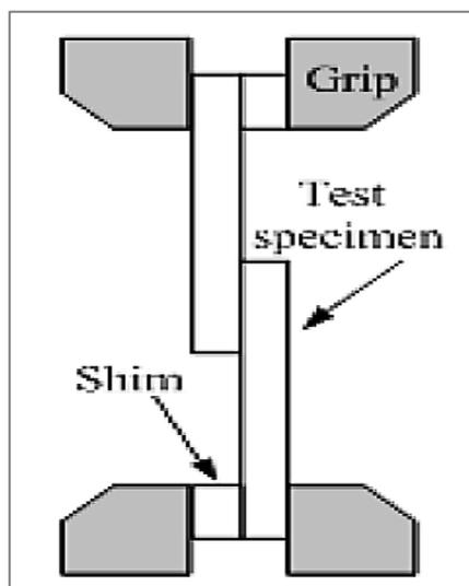
Figure 6: Schematic of a tensile strength test
