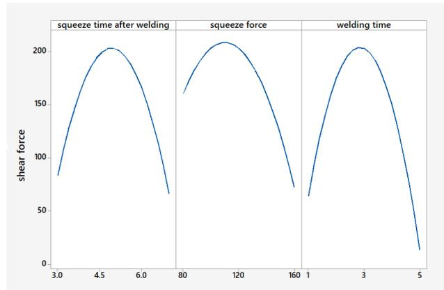
**Fig. 9: Perturbation of shear stress showing the effect of each input parameter over the selected level.**
