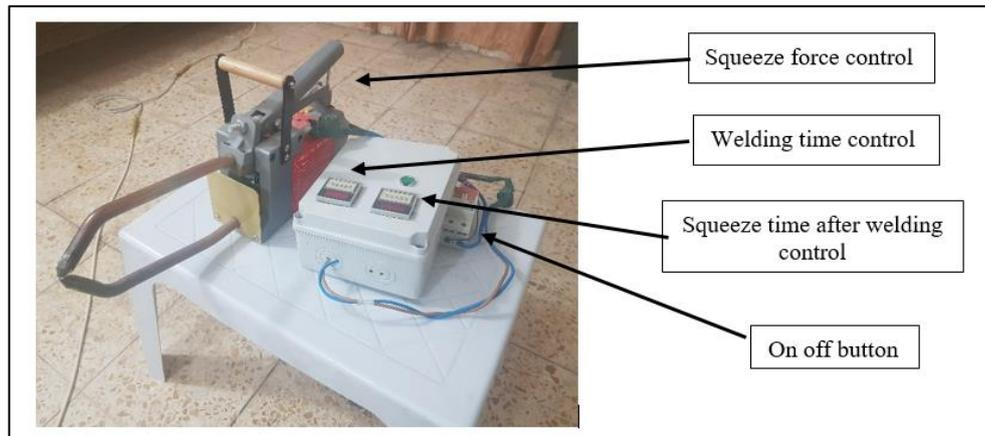
Figure2. Resistance spot welding machine.
