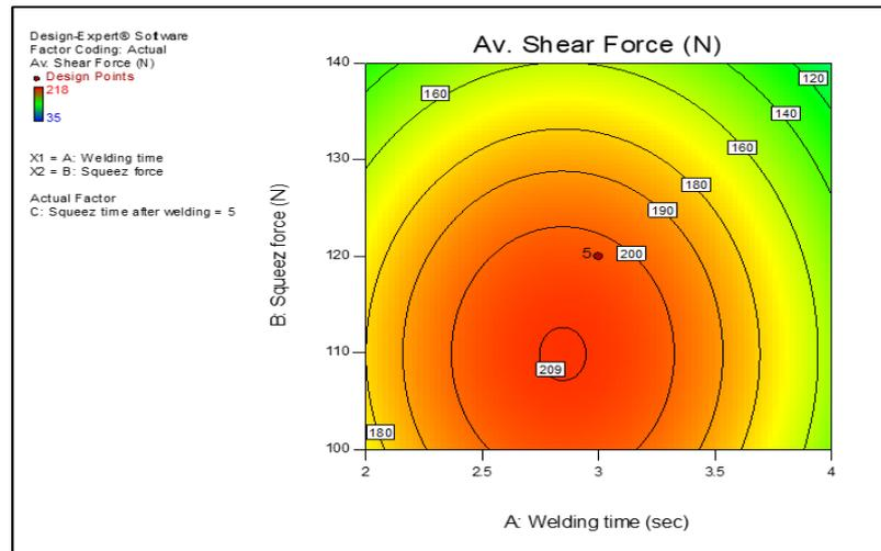
**Fig.10: Contour graph of shear force as a function of welding time and squeeze force.**
