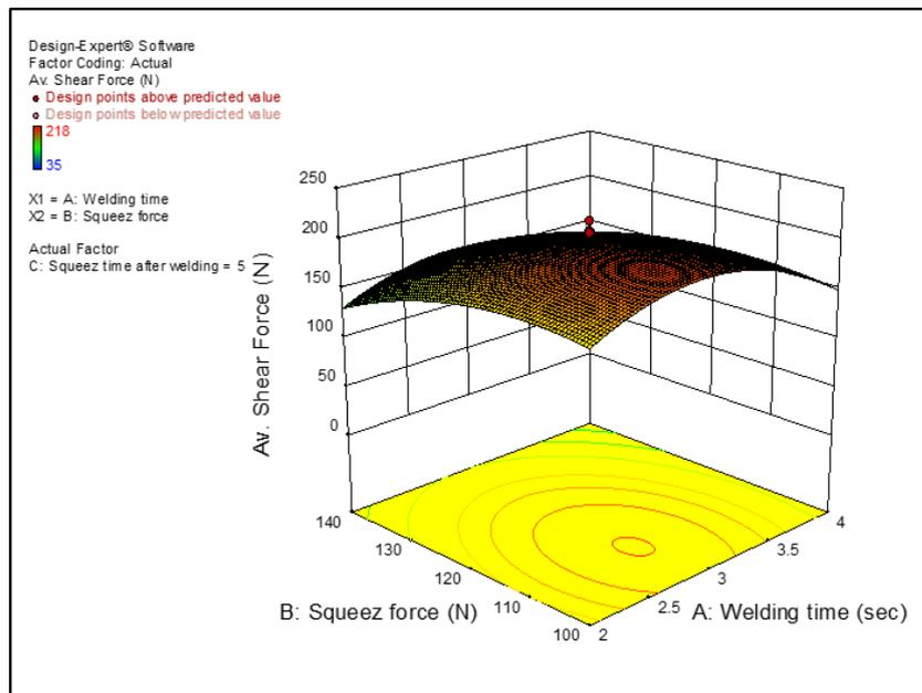
**Fig.11: 3D Graph of shear force as a function of welding time and squeeze force**
