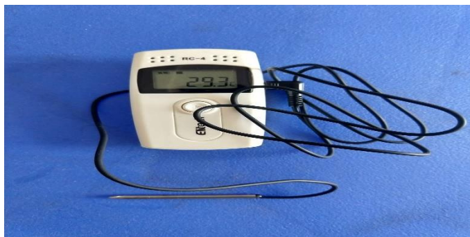
Figure 1: Temperature data logger
