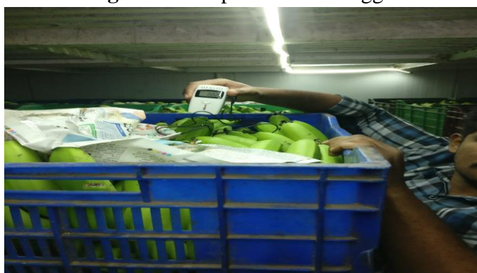
Figure 2: Inserting the temperature probe of data logger into the banana for data logging in the ripening chamber
