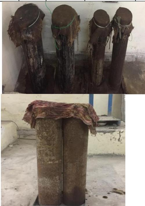
**Fig. 3** Circular concrete filled steel tube columns closed with wet burlap for curing
