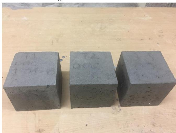
**Fig. 1** Concrete cube specimens
