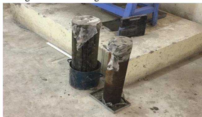
**Fig. 2** Circular concrete filled steel tube columns closed with a plastic sheet
