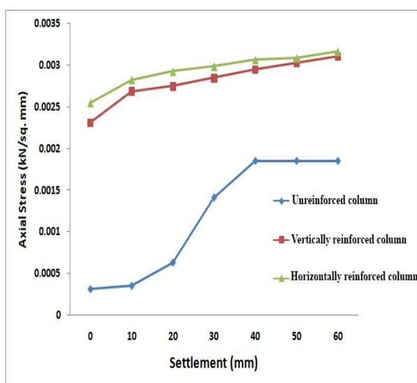
(b) Variation of axial stress versus settlement from the model testing
