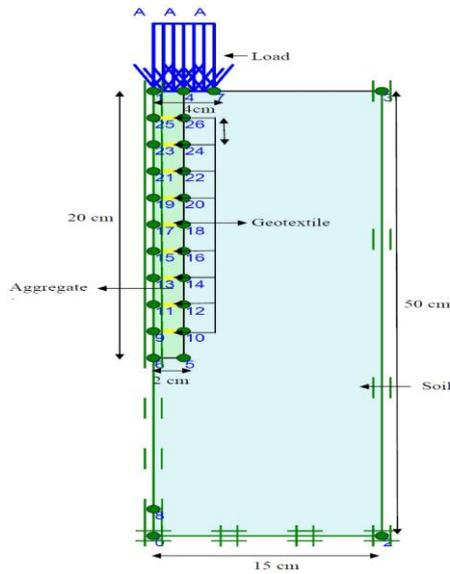
(c.) Geometry of model having structural elements in all.
