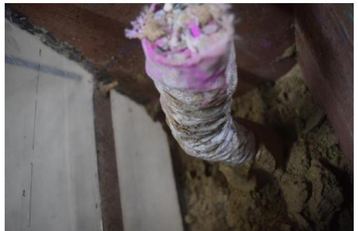
(c). Vertical reinforcement column failure due to bulging
