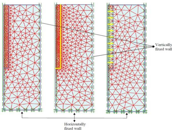
**Fig. 7.** Generated Initial Mesh
