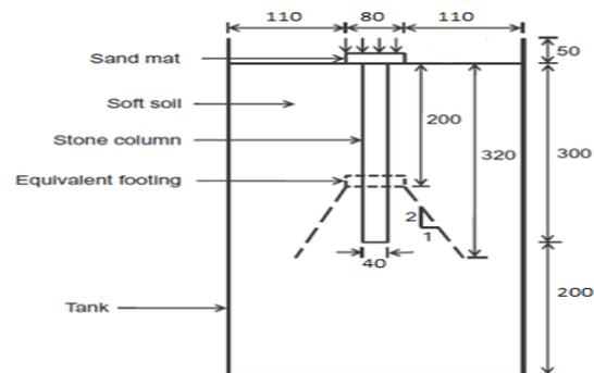
**Fig. 3.** Isolated stone column Schematic view
