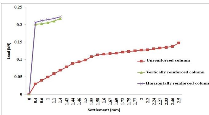
Fig. 9. Behaviour of Load versus settlement from Plaxis 2D
