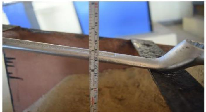
(b). Perpendicular distance measured from the column and the wall of modelled tank.
