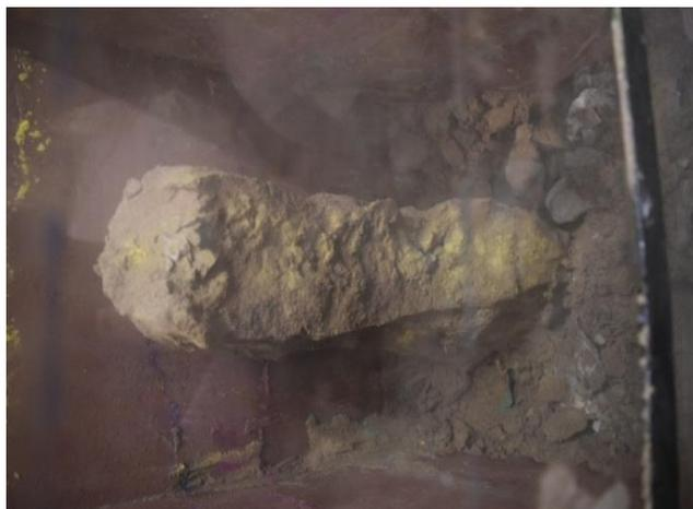
(d). Horizontal reinforcement column failure due to bulging.
