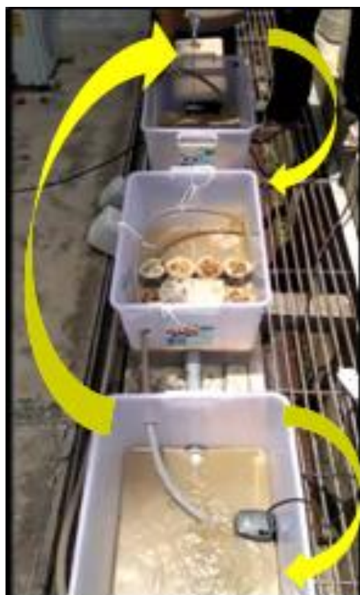
Fig. 3 Flow of leachate liquid in the filtration system C3
