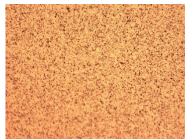
Figure 8. PCD surface after WEDM process (x200)
