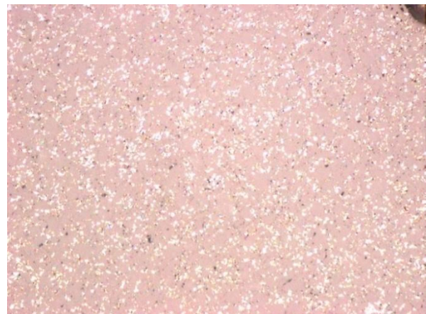
Figure 12. WEDM process PCD surface with agent preventing electrolyte exposure (x500)
