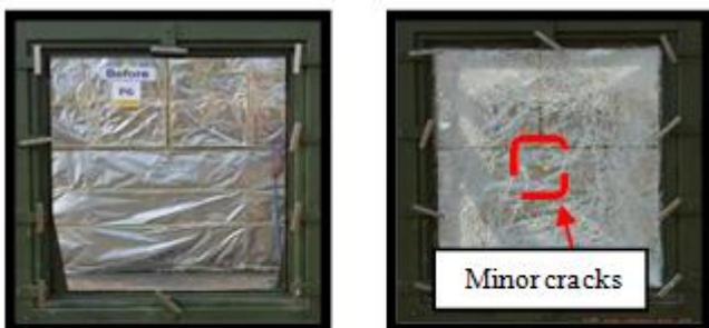
**(a) Before blast test (b) After blast test Figure 8 Laminated glass with SGP interlayer before and after the blast tests**
