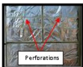
**Figure 7 Perforations of laminated glass with PVB interlayer**
