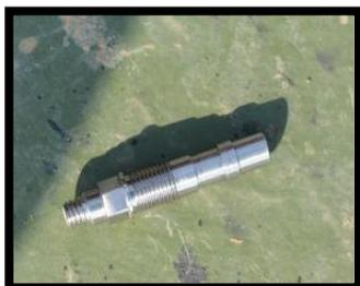
Figure 3 Piezoelectric pressure sensor
