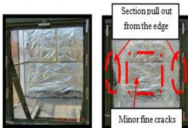
(a) Before blast test (b) After blast test
