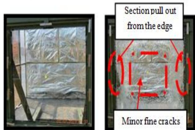
**(a) Before blast test (b) After blast test Figure 6 Laminated glass with PVB interlayer**
