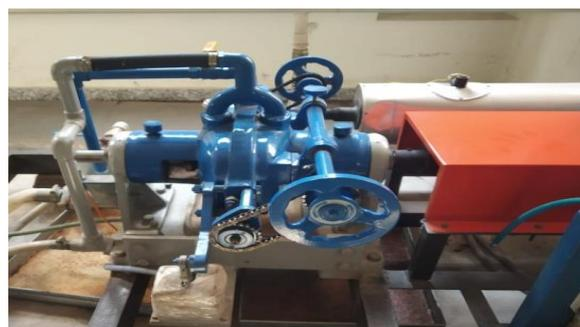
**Figure 3:-Hydraulic Dynamometer**
