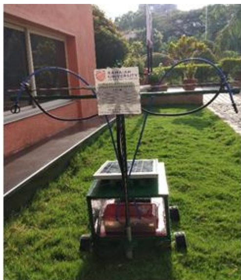
Fig. 10: Three DoF spraying Robot on Lawn
