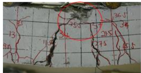
Fig. 5: Concrete crushing failure on BC1
