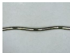
Fig. 2 Brass plated tire steel cord
