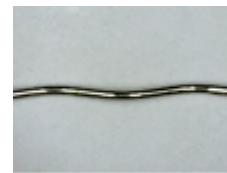
Fig. 2 Brass plated tire steel cord
