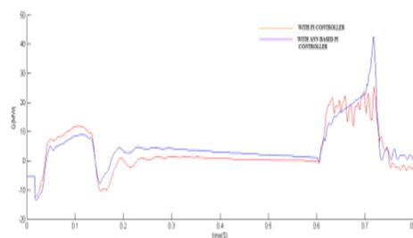
**FIG.8 Comparison of Real and Reactive Power with PI and ANN based PI Controller during LLLG Fault.**
