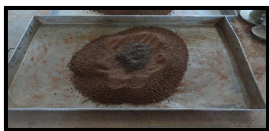
Fig. 3 Replacement of Sand with Iron Slag.
