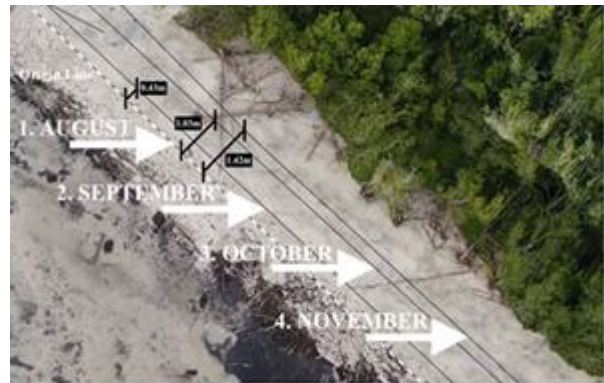
Figure 11: The shoreline during high tide represented by lines of the consecutive four months
