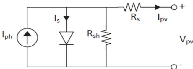
Fig. 2 .PV panel model with one diode
