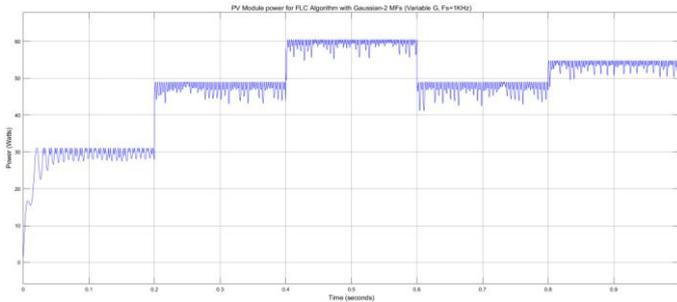
Fig. 15. Power waveform of PV panel with gaussian-2 MF.
