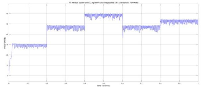
Fig. 11. Power waveform of PV panel with trapezoidal MF.
