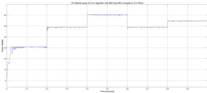
Fig. 9. Power waveform of PV panel with bell type MF.
