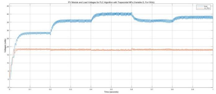
Fig. 12. Voltages of Boost converter at input and output.
