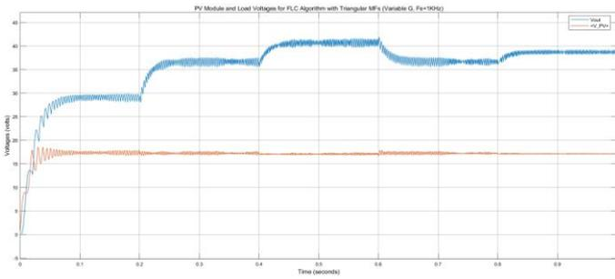
Fig. 8. Voltage waveform at converter input and output stages.
