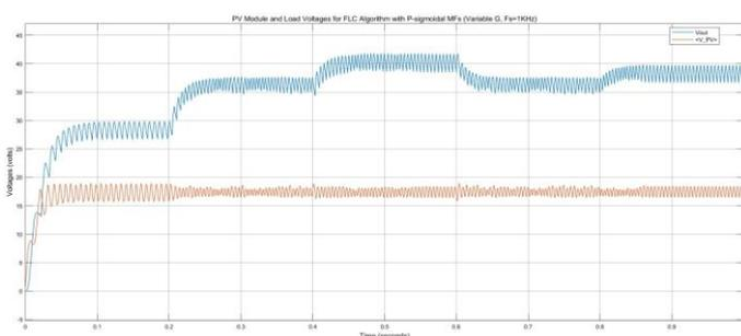
Fig. 18. Input and output voltages of Boost converter.
