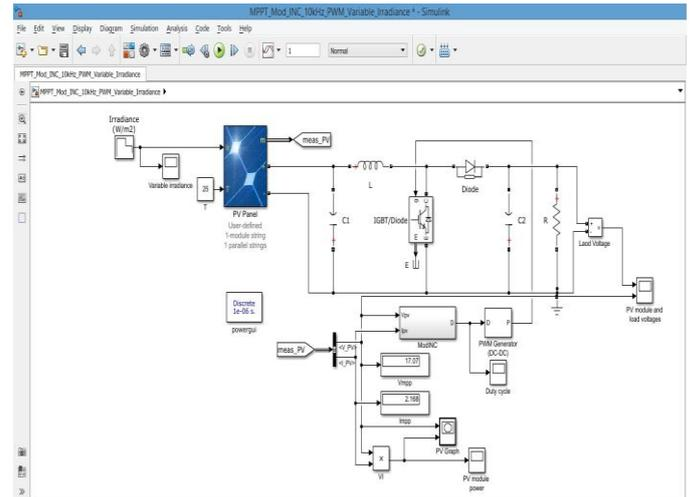
Fig. 5. PV system Simulink diagram.
