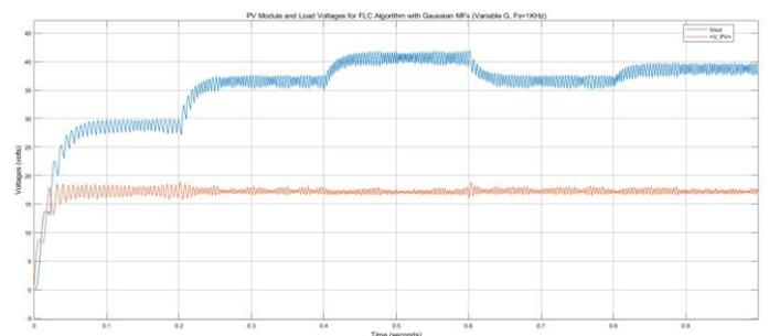
Fig. 14. Voltages of Boost converter at input and output.
