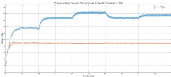
Fig. 10. Voltage waveform at converter input and output stages.
