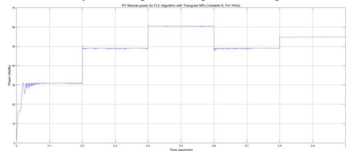
Fig. 7. Power waveform of PV panel with triangular MF.
