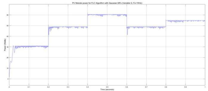
Fig. 13. Power waveform of PV panel with gaussian MF.
