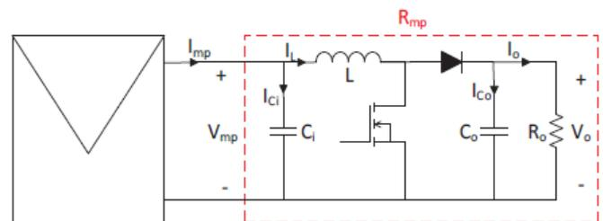
Fig. 4. Boost converter electric circuit.
