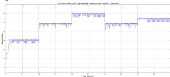
Fig. 17. Power waveform of PV panel with P-sigmoidal MF.
