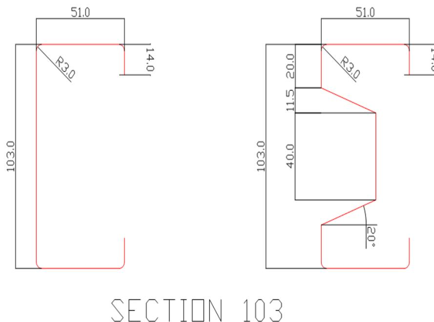
Figure 1: Cross section shape and dimensions of C-sections and  $\Sigma$ -sections
