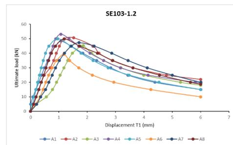
**Figure 4: Load-displacement curve for columns SE103-1.2**
