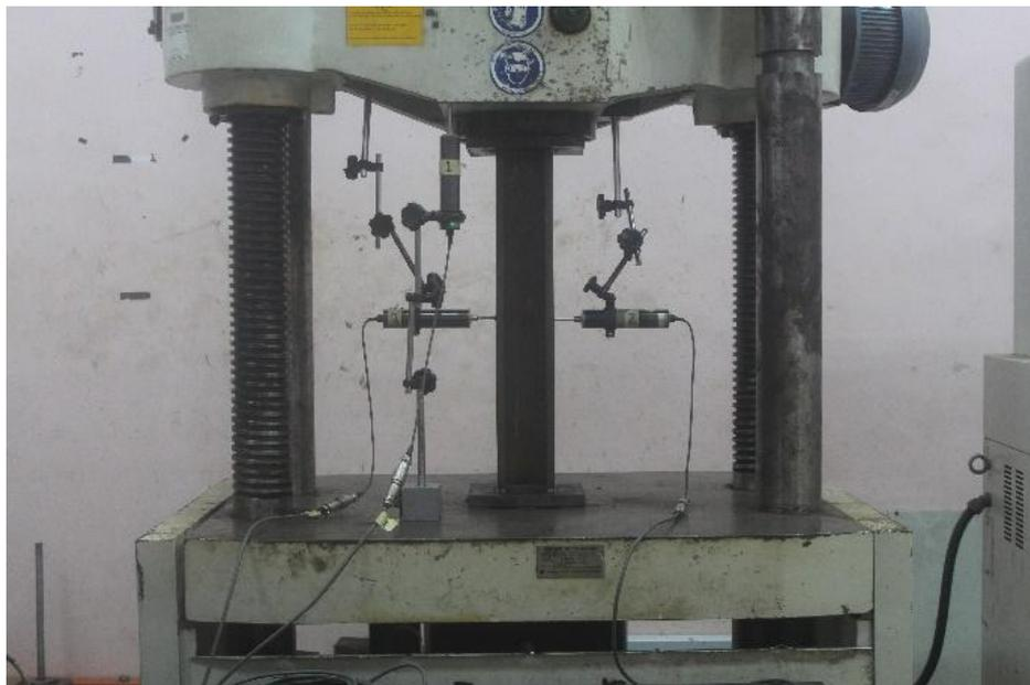
Figure 3: Short column test set-up and instrumentation
