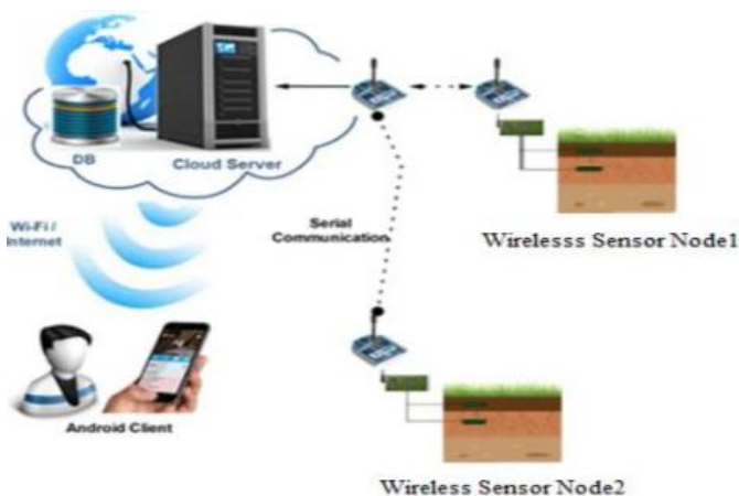
Fig. 2 smart irrigation using Zigbee
