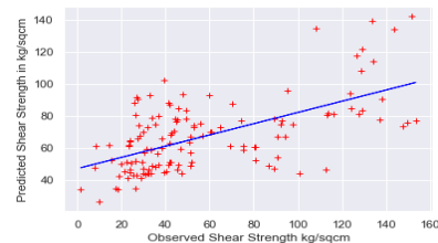
Fig. 8. association figure of observed with predicted values of Shear Strength of MLP Model
