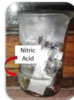
Figure 4. Pharmaceutical Blister packaging Separation Process
