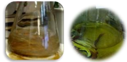
Figure 2. and Figure 3. Pharmaceutical Blister Packaging separation result with mix solvent (Sulfuric Acid 95% + Nitric Acid 65%)
