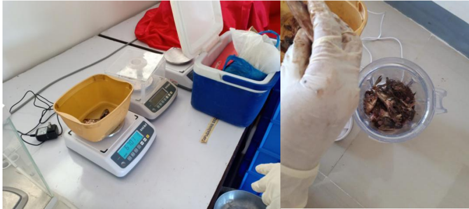
Figure A.1. Weighing and preparation of fish waste for homogenization (April 24, 2019 at PSHS-CMC Biology Laboratory )
