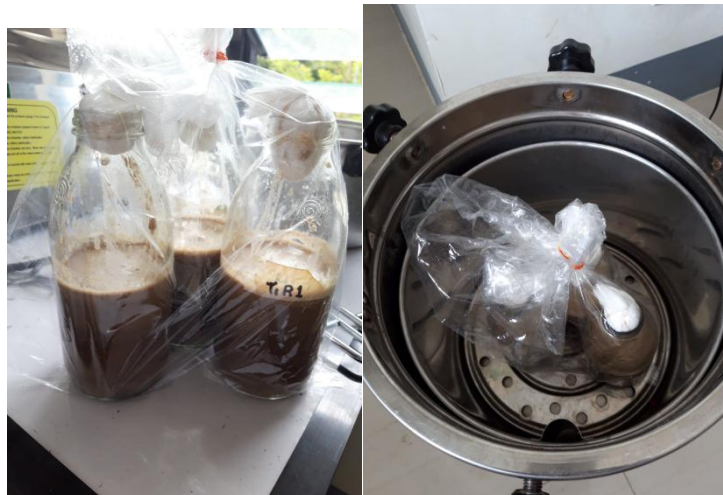
Figure B.2. Performing of acid hydrolysis in an autoclave at 15 psi and 121 degrees Celsius for 90 minutes (April 24, 2019 at PSHS-CMC Biology Laboratory)
