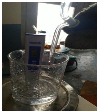
Fig 9.3.1 Alkalinity test of water sample
