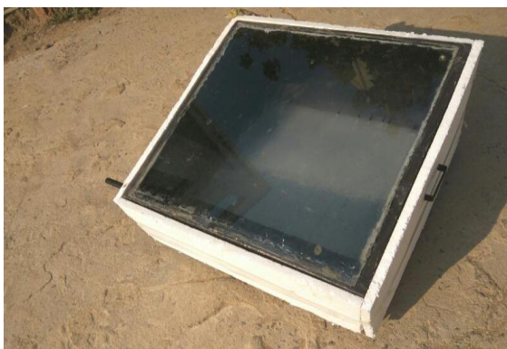
Fig 2. Conventional single slope solar still
