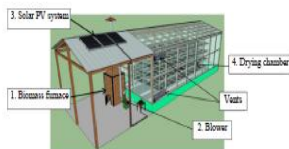
Figure 9 Solar-Biomass Hybrid Dryer
