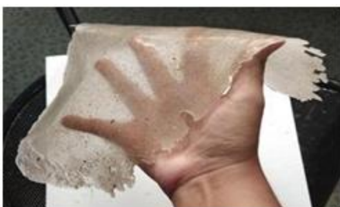
Fig.5: Fibers with Epoxy Resin (Less Hardener)
