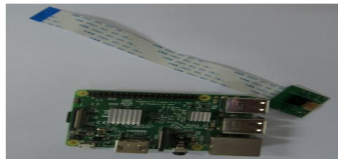
Fig. 3: Raspberry Pi 3B and Pi-Camera
